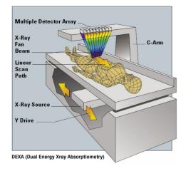
and the other by bone. The soft tissue amount can be subtracted from the total and what remains is patients bone mineral density. The DXA machines feature a special software that compute and display the bone density measurements on computer monitor.
