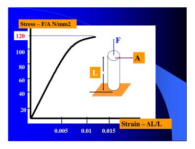
The ratio of stress to strain in the initial linear portion is the <u>Young's</u> <u>modulus</u>, that is:
